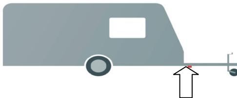
Next, push the stabilization pipes as far from each other as possible, towards the sides of the side members. Tighten the right and left fittings so that the bent underside of the fittings is positioned precisely against the outer side of the side members. Make sure that the bolts are tightened to the maximum extent.
