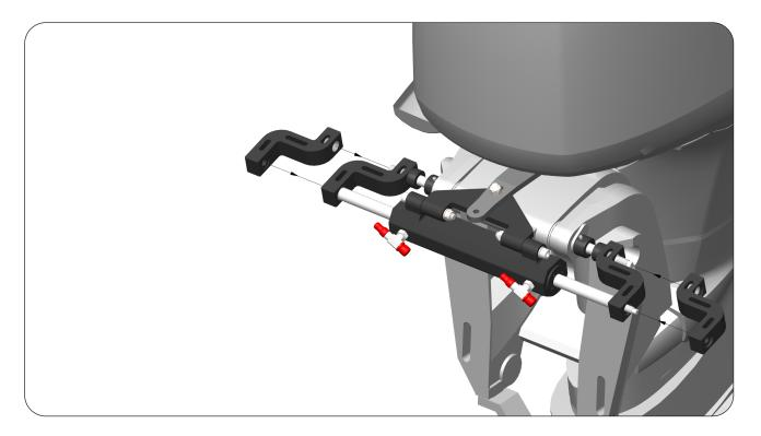
**STEP 9 :** Insert the Washers (10) and Nyloc Nut (11 & 12) on the two ends of the Support Rod (3) & Piston Rod (1) respectively. Grease the Nyloc Nut threads with any Anti-Seize Grease. Tighten first the Center Shaft Nuts and then Piston Rod Nut by using a 19 mm Wrench with a torque of 70 Nm (52 lb ft).
