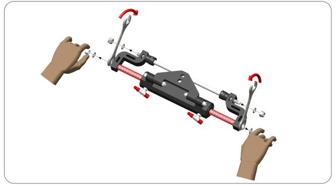
**STEP 2 :** Disassemble the Cylinder by removing Support Brackets (4), Delrin Washer Small (7), Delrin Spacer Big (6), Mounting Spacer (8) & Washer (10).
