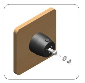
**STEP 1 :** Remove the Nylock Nut (6) & Washer (8) from the Helm Shaft.
