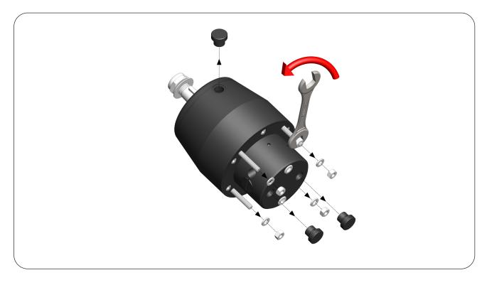
**STEP 5 :** Insert and tighten by hand the Elbow Fittings (1) until they are fully seated, then tighten with a wrench. Turning again from 1.5 to 2.5 turns, for their best orientation for the Hose connection. However do not exceed a maximum torque of 17.6 Nm (13 lb ft). Also insert the Oil Filling Plug with Breather Hole (2) into Oil Filling Port
