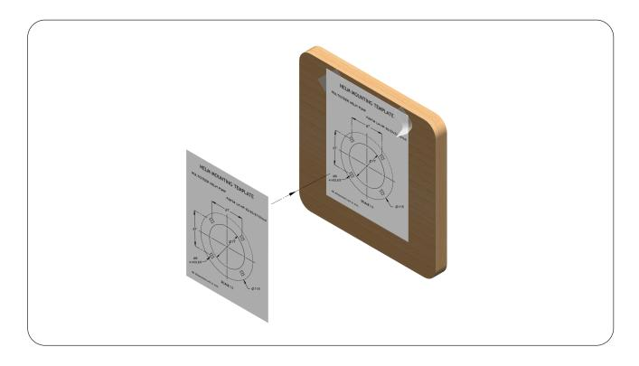
**STEP 3 :** Make 4 holes for the flange studs with the help of a Hand Drill and a big one for the center hole with the help of hole saw.
