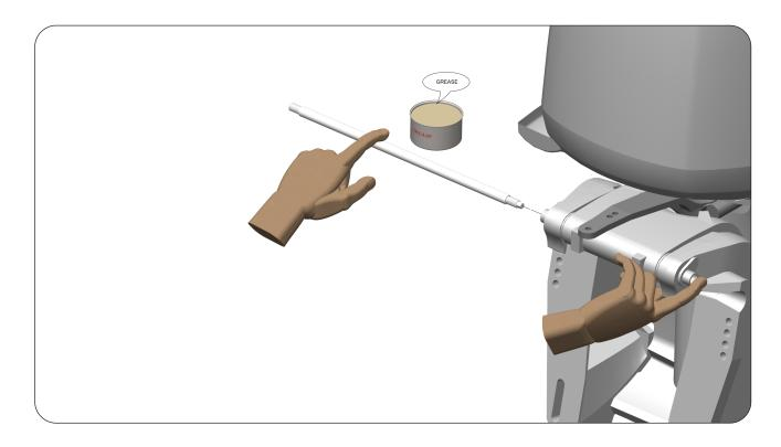
**STEP 4:** Assemble the Tiller Hex Stud Assembly (5) into the Tiller Plate (2) of Cylinder as shown.
