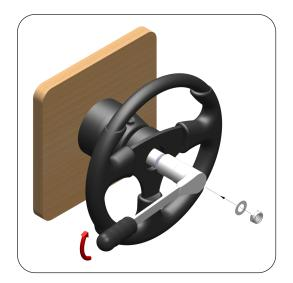
**STEP 3 :** Fit the Steering Wheel on the Shaft by inserting the Specific Key (4) in its compartment. Insert the Washer (8) and use a 20mm Hexagonal Wrench to tighten the Self-Locking Nut (6) with a 40 Nm (29.5 lb ft) torque.
