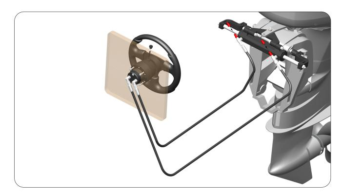
**STEP 18 :** After tightening the Oil Filling Plug, some amount of Oil will come out around the plug for some period of time when the Wheel is turned lock to lock. This Oil seepage will be over when the system is stabilized and no air is trapped inside the system.
