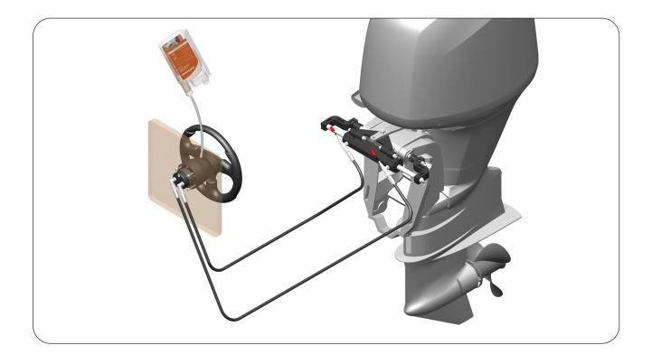
**STEP 12 :** Insert the other pipe supplied with the Cylinder into the air bleeders for collecting the Oil, coming out from the air bleeders during purging process.
