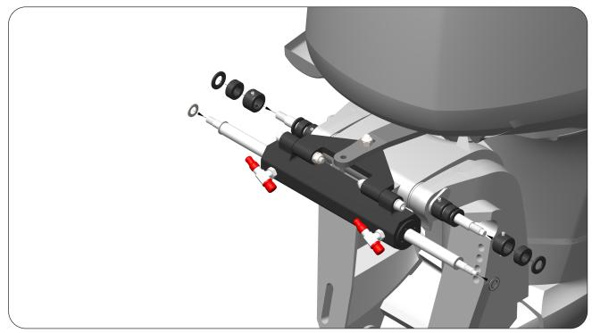
**STEP 8 :** Insert the right and left Support Brackets (4) by connecting both the Piston (1) & Support Rods (3) as shown in the picture.
