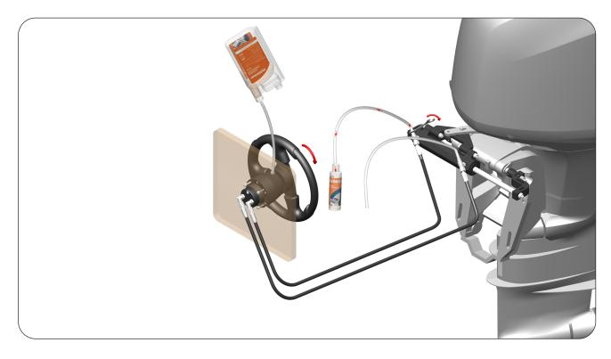
**STEP 16 :** Continue to turn the Steering Wheel towards Port Side. When the Oil comes out from air bleeder without air bubbles then carefully close the air bleeder. Do not overtight more than 15 Nm the air bleeder. Continue to turn the Steering Wheel in the same direction to fill the Cylinder chamber. During this phase the Cylinder body will move to the opposite direction up to the end stroke.
