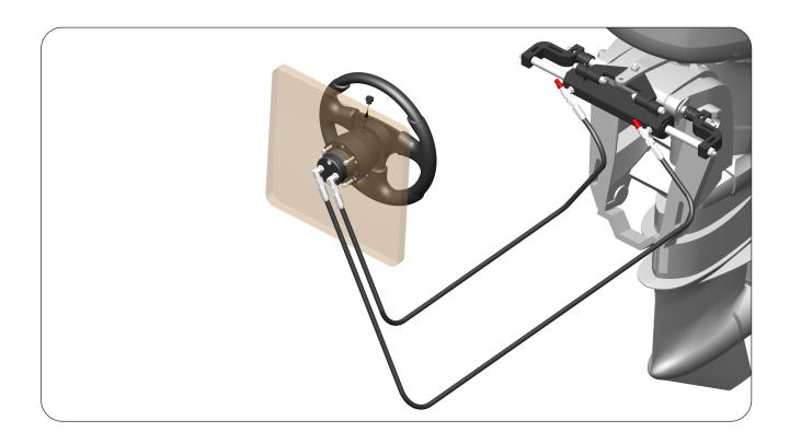
**STEP 10 :** Insert the threaded port of pipe into the Oil Filling Port of Helm. Turn the bottle upside down and carefully remove the other side of cap to ease the Oil passage towards the Helm. Fill the Helm until no air bubbles are visible in the pipe.
