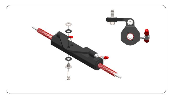
**STEP 5 :** Position the Engine straight so that its Engine Arm is perpendicular to the Transom. Connect the Tiller Arm (2) of Cylinder to the Engine Arm by means of the Hex Stud (5). Tighten it by using a 14mm Wrench with a torque of 20 Nm (14.75 lb ft). Tighten the Nyloc Nut of Hex Stud by using a 14mm Wrench with a torque of 20 Nm (14.75 lb ft). After tightening the Nyloc Nut, check for the right torque 20 Nm (14.75 lb ft) of the Hex Stud (5).
