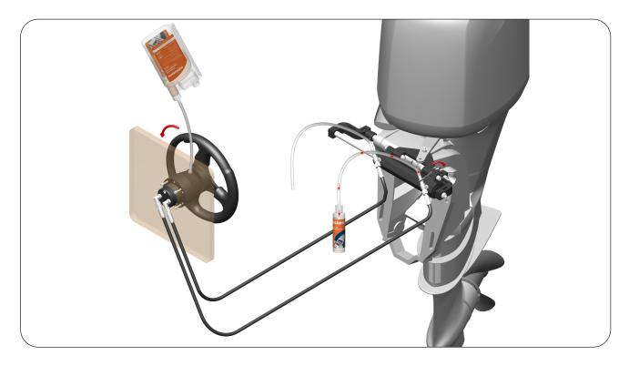
**STEP 14 :** Continue to turn the Steering Wheel towards Starboard Side. When the Oil comes out from air bleeder without air bubbles then carefully close the air bleeder. Do not overtight the air bleeder. Continue to turn the Steering Wheel in the same direction to fill the Cylinder chamber. During this phase, the Cylinder body will move to the opposite direction up to the end stroke.
