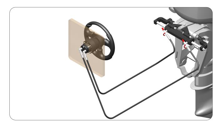
**STEP 6 :** Ensure that all the Hose Fittings should be tighten properly. Hoses should not be bent in excess. Minimum Hose bent radius is 100 mm (4 Inch). Ensure that there should be no interference during engine tilting as well as no interference with the transom.
