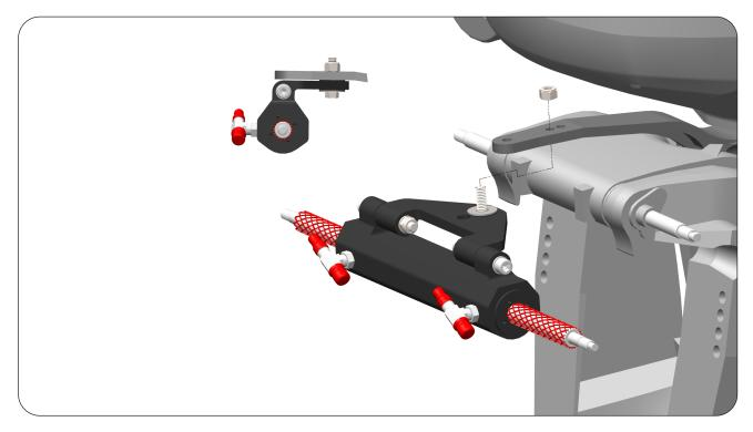
STEP 6: Remove the Piston Rod Protector before assembling the Support Bracket (4).
