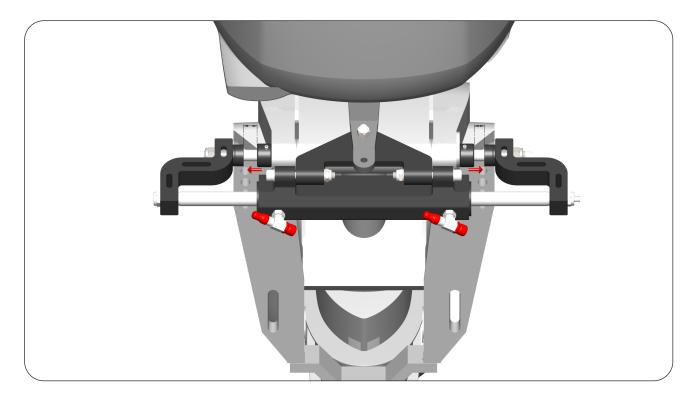
**STEP 11 :** Verify if the Cylinder installation is correct by manually moving the engine on the Starboard & Port side. The displacement must be as symmetric as much as possible between Port and Starboard so that the Steering angle is the same on both sides.
