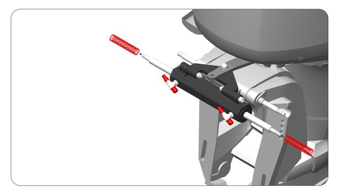
**STEP 7 :** Insert the Mounting Spacer (8), Delrin Spacer Big (6), Delrin Washer Small (7) & Washer (10) as show. With reference to the "Application Guide" Choose the correct number of washers for the tilt tube rod. In this phase ensure that the Cylinder body is centered on the Piston Rod (1) and that the Engine is perpendicular to the Transom.
