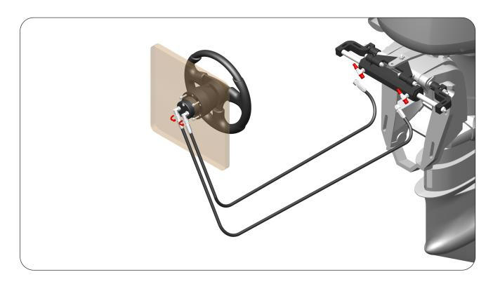
**STEP 4:** Remove the thread protector caps from both the T-Fitting Hose Side Port of Cylinder.
