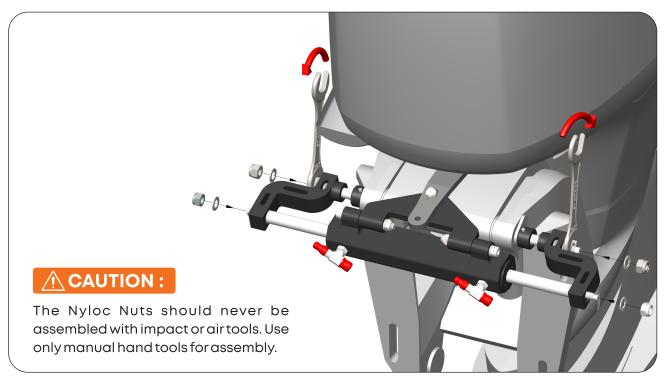
**STEP 10 :** Adjust the space on the Tilt Tube with the help of tightening the Mounting Spacers (8) until the clearance is eliminated.
