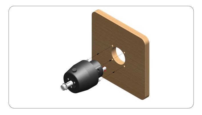
**STEP 7 :** Tighten the 4 Hex Nuts (7) & the 4 Washers (9) through the Flange Studs (5) of the Helm to the dashboard with the help of a 10mm Wrench with the torque of a 10 Nm (7.4 lb ft).
