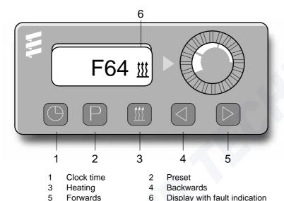
If the control unit detects a fault when the heater is switched on or while the heater is in operation, the timer module indicates this by means of an F and as a 2-figure number within 15 seconds.
